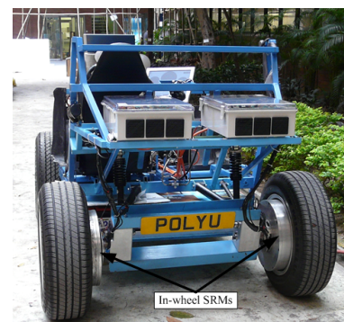
EV prototype driven by in-wheel SRMs
